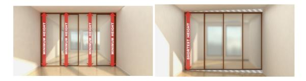
7. It is not common, but if your floor and ceiling are both not level and are running out in the same direction, you must calculate the opening height using the shortest levelled height as shown below. If you believe you have this type of space and need support, you can contact us any time, 24/7, 365 days per year and we will assist you.
