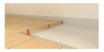
5. Now you can measure the width of the opening in mm in a minimum of 4 places. You should measure the top, the bottom and as many places as you can between and make a note of the smallest of the measurements taken.
