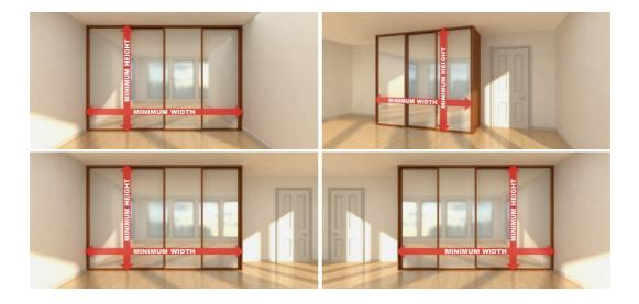
4. You should now consider what floor finish you have and whether the bottom track and casing will be fixed directly to the floor finish or whether the floor finish will be removed first. If you plan to remove the floor finish prior to fitting the bottom track and casing, please allow for this when you take your opening height measurements.
