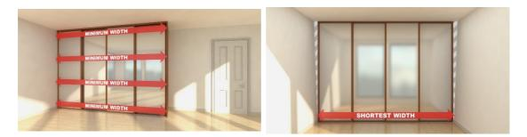
6. You can now measure the height of the opening in mm in a minimum of 4 places from the ceiling to the floor surface the wardrobe will be fitted to. You should measure the left hand side, the right hand side and as many places as you can between and make a note of the smallest of the measurements taken.
