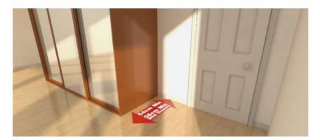
3. When measuring the wardrobe opening, please ignore any skirting boards, dado rails, picture rails or cornices and simply measure from ceiling to floor and from the outer left hand edge of the opening to the outer right hand edge of the opening whether that be wall to wall, wall to outside of end panel or outside of end panel to outside of end panel.
